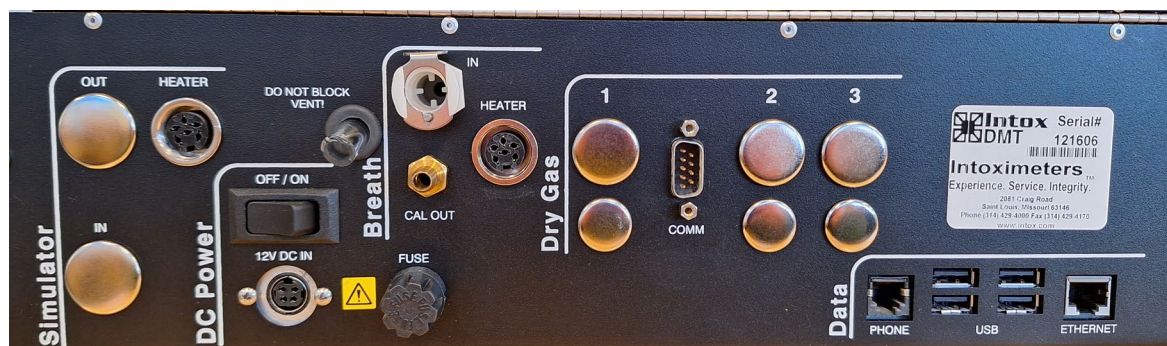
Figure 6. Back panel view of the DMT
